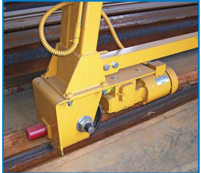
Spanco Guide Angle Drive Kit with Guide Rollers.
