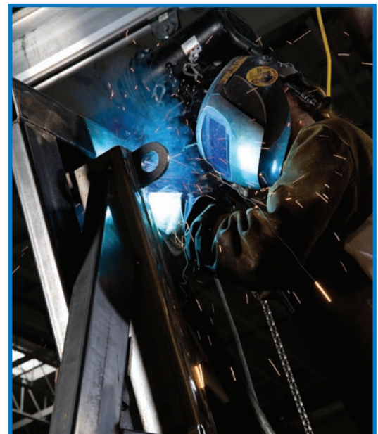
A Spanco worker in Las Vegas welding the A-frame on an Aluminum Gantry Crane.
