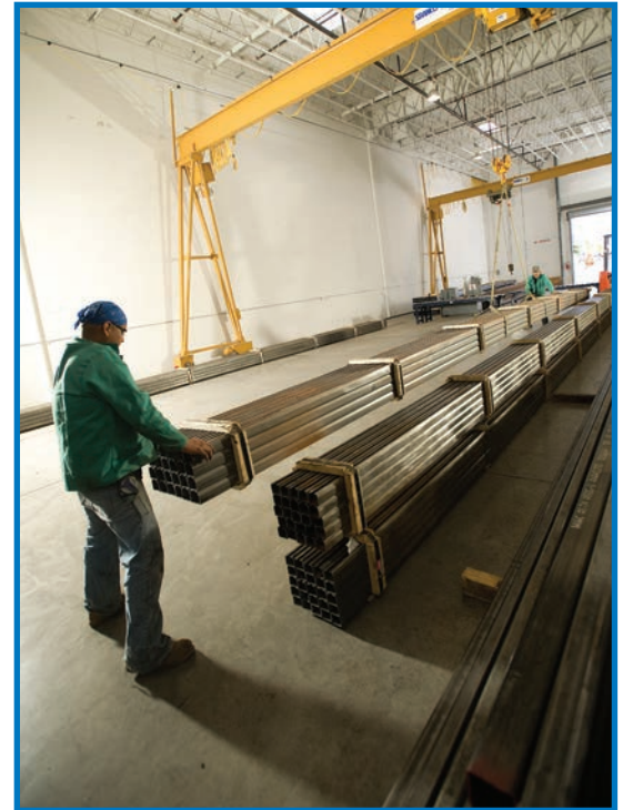
Workers using two Motorized Spanco PF-Series Gantry Cranes to load and transfer steel bundles.
