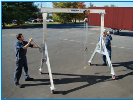
Two workers adjusting the height on an aluminum gantry crane using a Lug-All® Winch Hoist.
