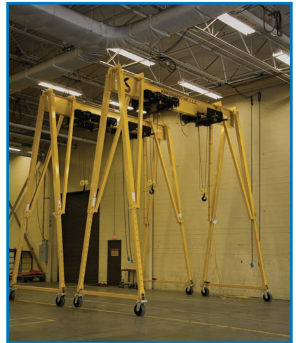
Dual Spanco T-Series Gantry Cranes
