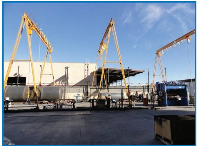
Three track-mounted PF-Series Gantry Cranes mounted over rail cars for easy maintenance and repair. The track mount ensures smooth travel over a fixed route for increased productivity and ease-of-use.
