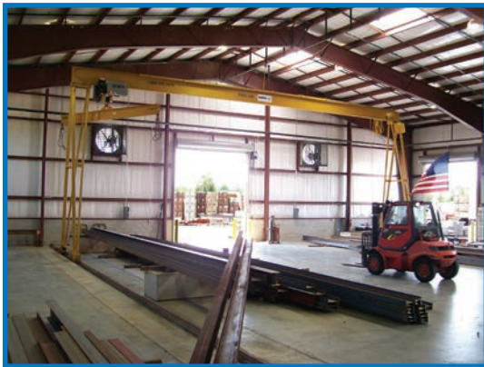
A Spanco Motorized 7.5-ton PF-Series Gantry Crane used to move truckloads of long steel beams at a building material supply center
